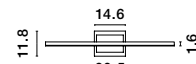
AZURE - 9267018 Sandy Black Aluminium & Acrylic LED 12.5 Watt 230 Volt 750Lm 3000K IP20 L:60.5 W: 6.9 H: 11.8 cm LED WARM WHITE DRIVER INCL.
