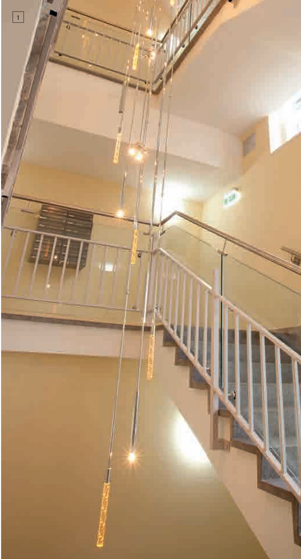
1 SA-DLU 2375/60/12+12/chrom/ Blase/LED-amber EEI + 5 x inner light Ø 60 cm, H 7,2 m 27 x G9/25 W (max. 40 W) + 12 x LED-1 W amber
