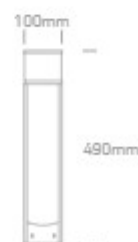
67494A | 3W | SMD LED | LED Bollard with 2xSchuko Sockets 1000W each | Die cast
