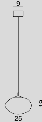
1653.1L SOSPENSIONE A ROSONE / HANGING LAMP WITH CANOPY Glass 1 x Ø 25 cm 1 x LED 6 W DIMM
